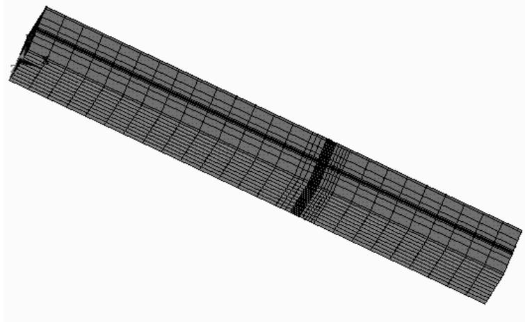
Fig. 2. Finite element discretization of the sandwich SCB
