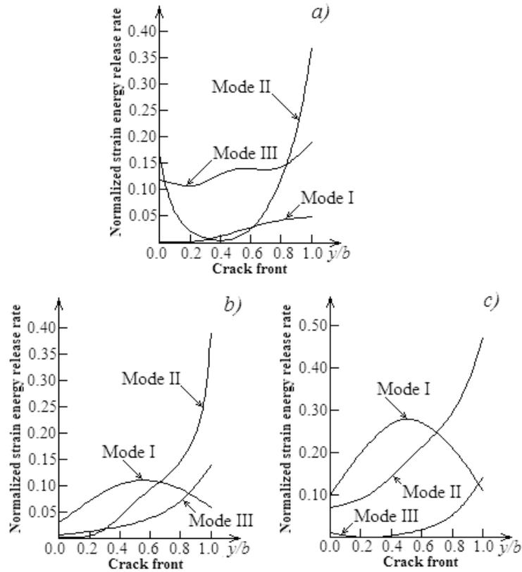
Fig. 6. Normalized strain energy release rate mode components distribution along the crack front in a sandwich SCB with relative crack length  $a/b_{of}$ : (a) 1, (b) 3, (c) 5. The imposed displacement magnitude is 18 mm. The horizontal axis is defined such that  $y/b = 0.0$  is at the left edge. Thus,  $y/b = 1.0$  is at the right edge. Here,  $b$  is the sandwich beam cross-section width
