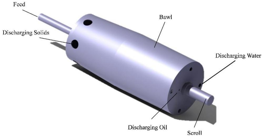
Fig. 1. (Color online) Schematic of a tricanter centrifuge.
