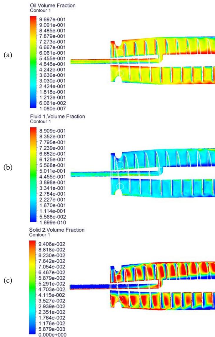
Fig. 5. (Color online) Volume fraction contour: Oil (a), Water (b), Solid materials (c).
