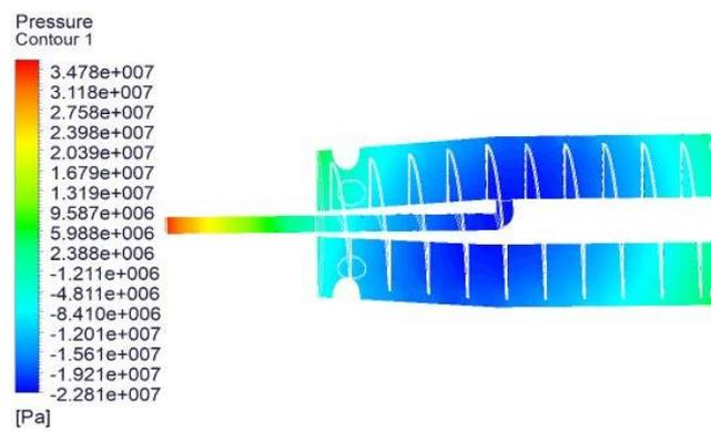
Fig. 4. (Color online) Pressure contour inside the tricanter machine.
