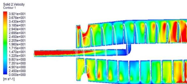
Fig. 3. (Color online) Solid materials velocity contour after the increase of the differential speed.
