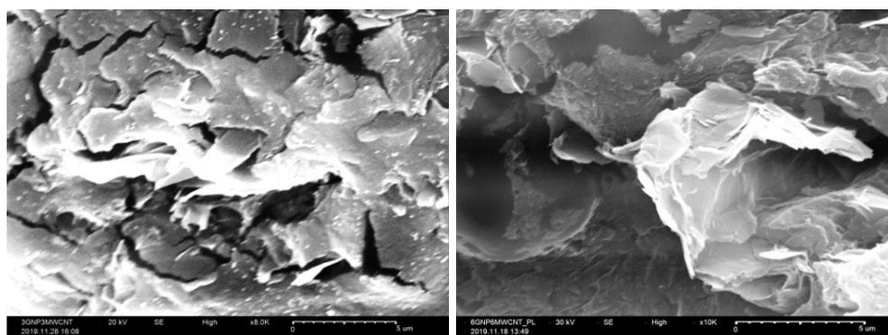
Fig. 6: SEM micrographs of 3 wt% GNP/3 wt% MWCNT/PLA (a) and 6 wt% GNP/6 wt% MWCNT/PLA (b) nanocomposites.
