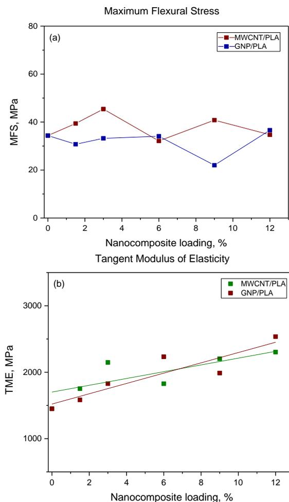
Fig. 3: Maximum flexural stress (a) and tangent modulus of elasticity (b) of PLA-based nanocomposites having single carbon filler in the hybrid structure.
