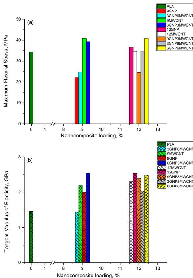
Fig. 5: Maximum flexural stress (a) and tangent modulus of elasticity (b) of GNP/MWCNT/PLA nanocomposites with overall 9 wt% and 12 wt% carbon loading.
