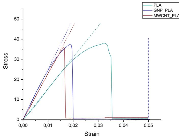
Fig. 2: Typical stress-strain curves showing different linear elastic portion and fracture point, respectively, for pure PLA, 12 wt% GNP/PLA and 12 wt% MWCNT/PLA nanocomposites.
