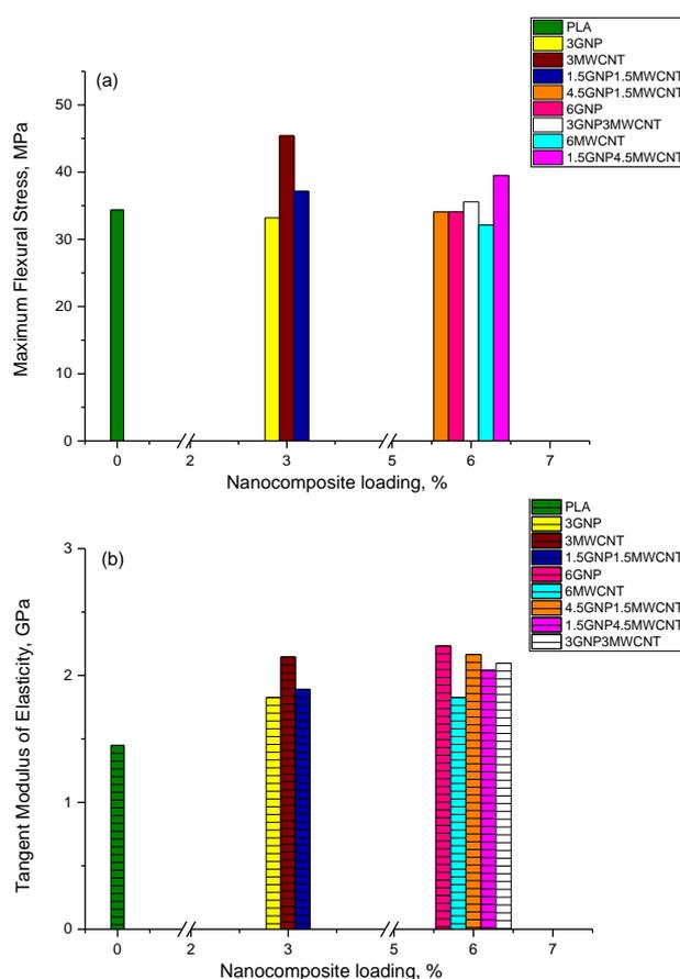
Fig. 4: Maximum flexural stress (a) and tangent modulus of elasticity (b) of GNP/MWCNT/PLA nanocomposites with overall 3 wt% and 6 wt% carbon loading.
