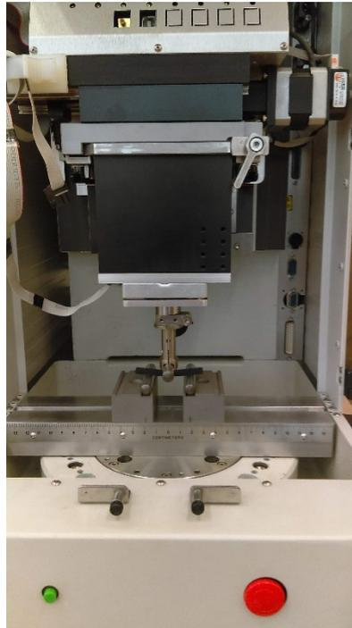
Fig. 1: Experimental set-up of three-point bending analysis using UMT-2 equipment.
