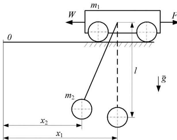
Fig. 1: A dynamic model of the system “crane trolley – load”.
