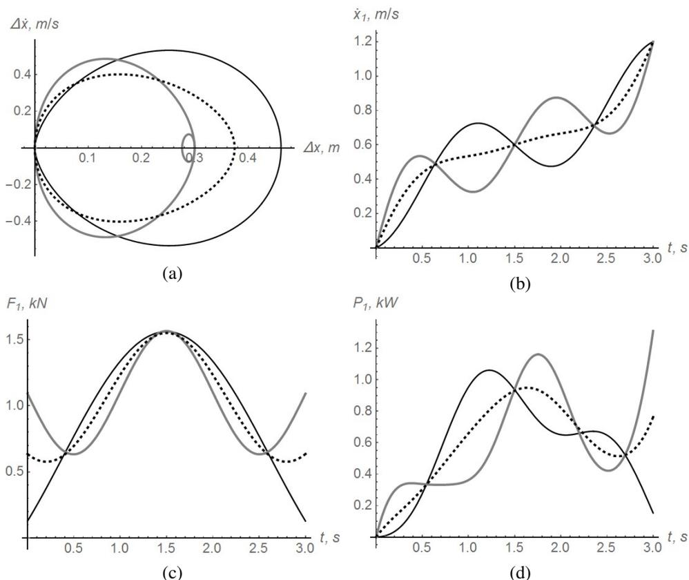
Fig. 2: Plots of the system's motion characteristics under the optimal control: (a) phase portrait of load's oscillations on the flexible suspension; (b) velocity of the trolley; (c) dynamic component of the drive force; (d) dynamic component of the drive power.
