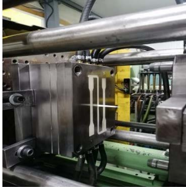
Fig. 1. Multipurpose specimens manufacturing from PA11 resin.
