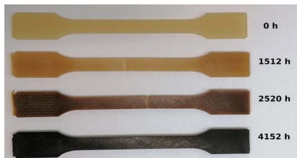
Fig. 3. Samples of PA11 exposed to accelerated aging at 125°.
