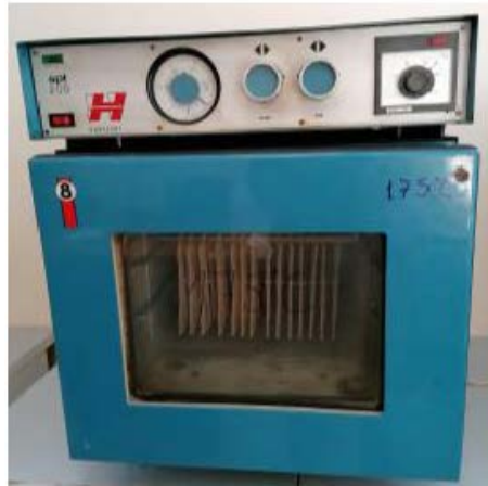
Fig. 2. Arrangement of specimens into drying oven.
