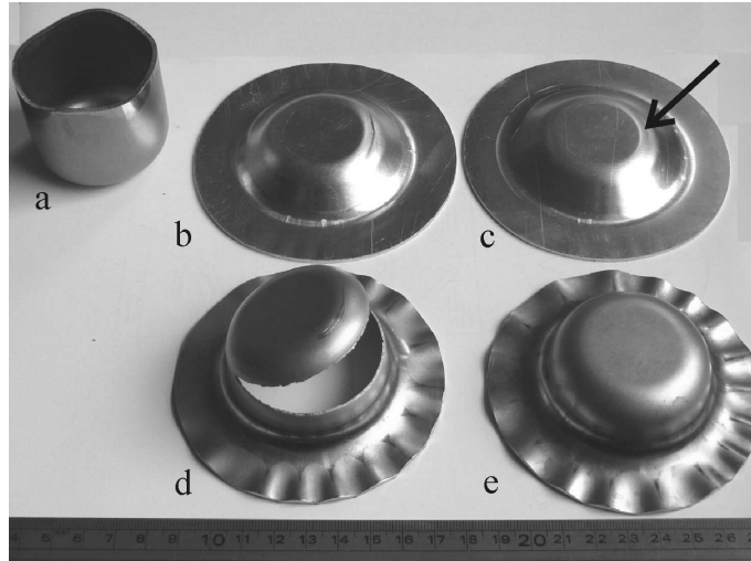
Fig. 4. Pieces obtained of deep drawing experiments: (a) Steel 08; (b, c) aluminium; (d, e) brass
