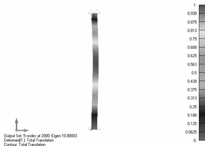
Fig. 7(b). Type “c-loading” configuration FEA results without the side loading
