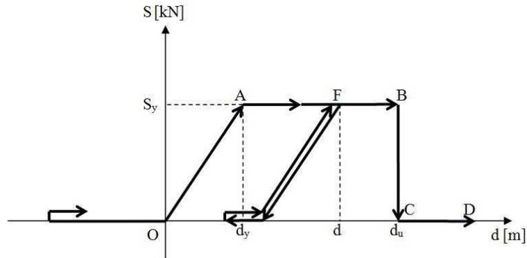
Fig. 4. The diagram for the constitutive law of cable-elements
