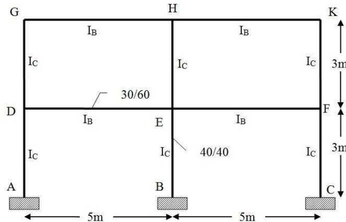
Fig. 1. The initial RC frame F0 without cable-strengthening
