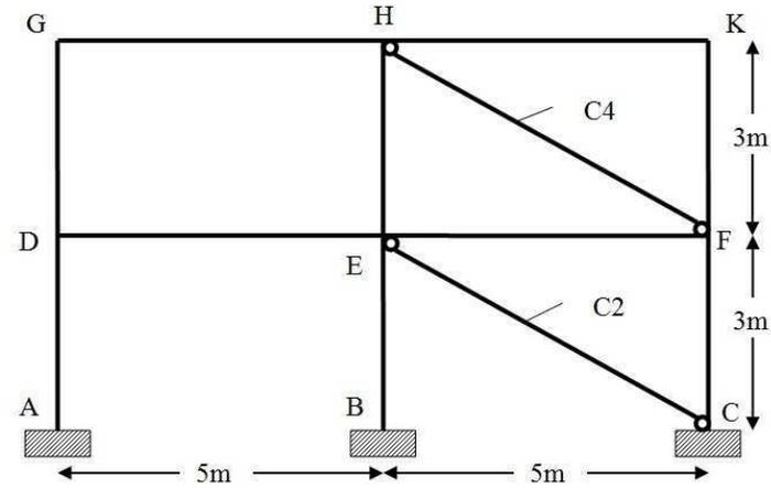
Fig. 2. The RC frame F1 with diagonal cable-strengthening
