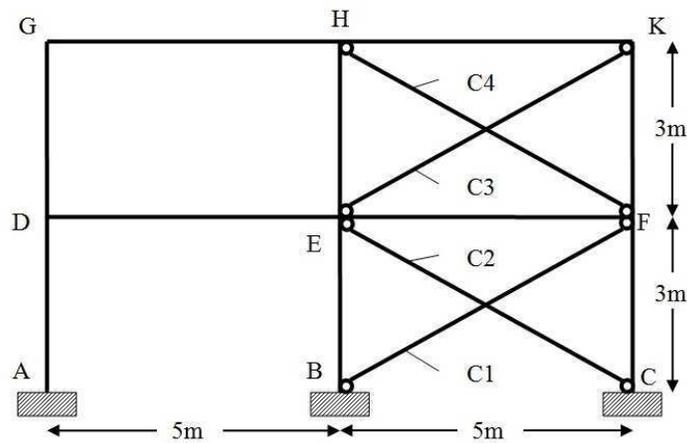
Fig. 3. The RC frame F2 with X-braces cable-strengthening
