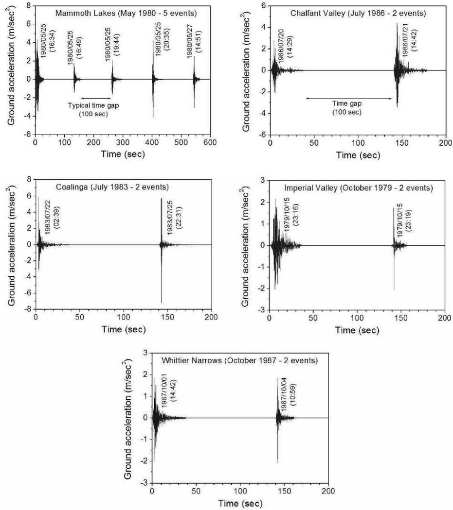
Fig. 5. Ground acceleration records of the simulated seismic sequences
