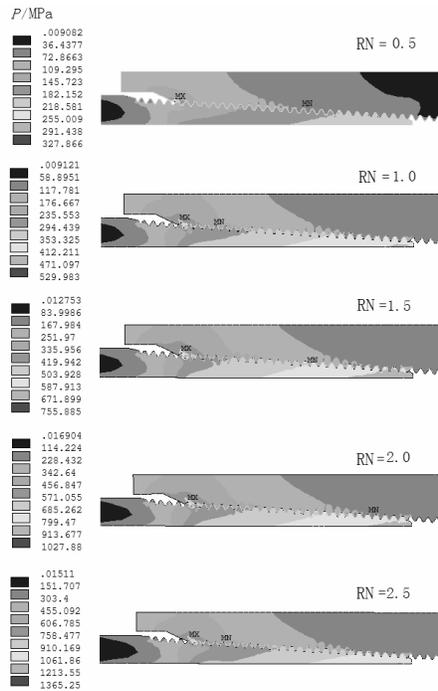
Fig. 9. Stress distribution cloud of coupling under different make-up torque
