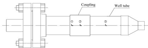
Fig. 5. The arrangement of measuring points
