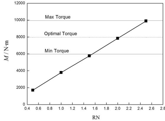
Fig. 10. Change relation between make-up torque and number of threads
