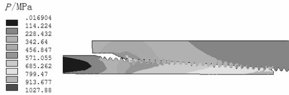
Fig. 7. Von-Mises stress distribution cloud of coupling
