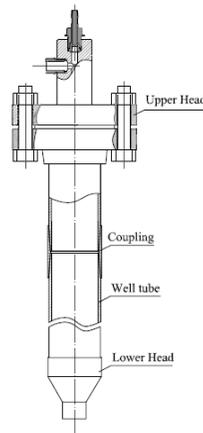
Fig. 1. Schematic diagram of structure for gas storage well
