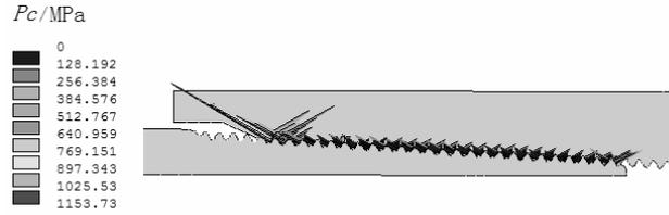
Fig. 8. Contact pressure distribution cloud of coupling
