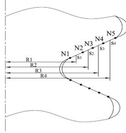
Fig. 6. Calculation schematic diagram of single-threaded torque
