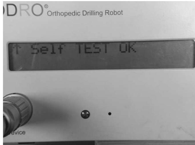
Fig. 6. The message on the display after positive result of the procedure 'Self Test'
