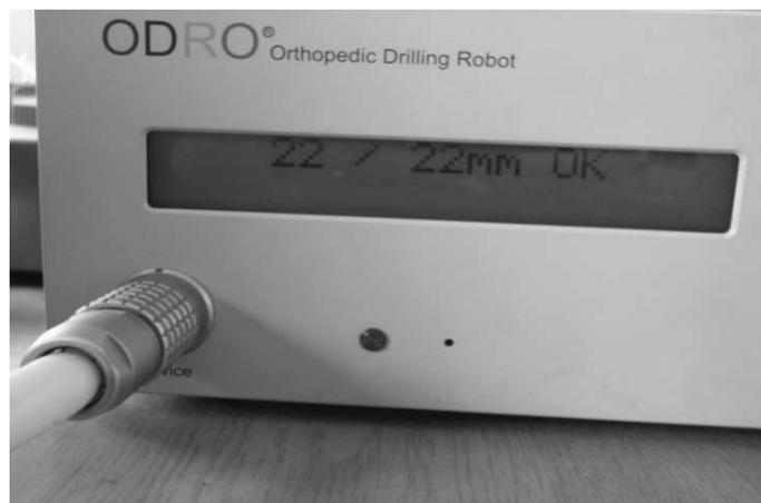
Fig. 3. Confirmation message after preliminary set depth drilling of 22 mm
