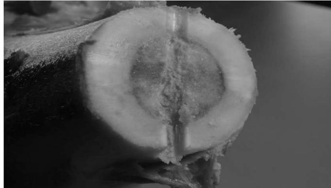
Fig. 5. Pork bone across cut section, after whole drilling with 6 mm drill bit diameter
