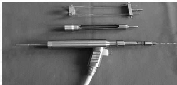
Fig. 1. Automatic drilling executive device and its accessories
