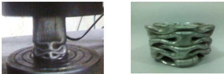
Fig. 8. Deformation pattern for the empty tube.
