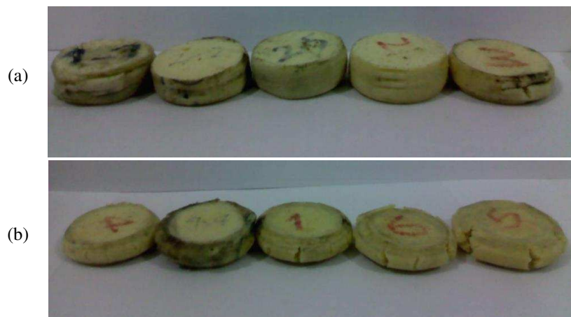
Fig. 3. Specimens after test in the experimental test: (a) from left to right, density is 80, 123, 147, 175 and 200 \text{kg/m}^3 ; (b) from left to right, density is 235, 251, 300, 350 and 400 \text{kg/m}^3 .
