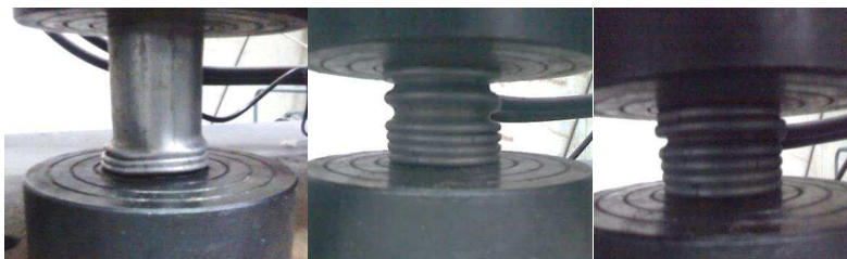
Fig. 9. Deformation pattern and crushing process for the FGF filled tube.
