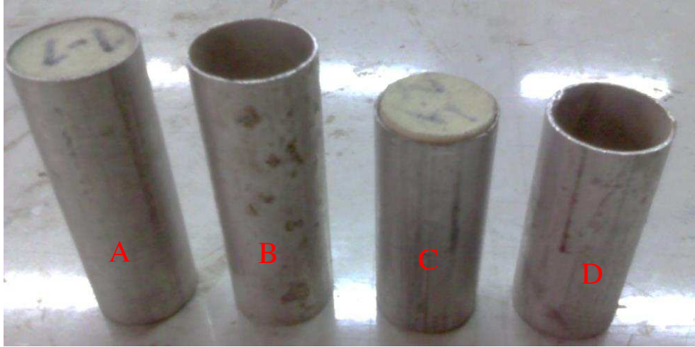
Fig. 7. First sample test with: (A) FGF filled tube; and (B) empty tube. Second sample test with: (C) FGF filled tube; and (D) empty tube.
