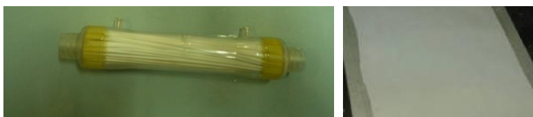
Fig. 1. (Color online) Visualization of hollow membranes (left) and flat sheet membrane (right).
