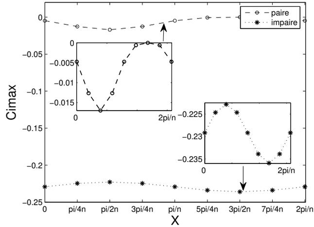
Fig. 8: Variation of the imaginary part of the most dangerous Odd and even eigenmode at different section  $x$  for SG fluid for  $\gamma = 0.01$  and  $Re_c$  corresponding of the most dangerous section.
