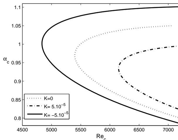
Fig. 5: Neutral stability curves for various values of the elasticity number  $K$  at  $\gamma = 0.03$  and  $x_c = 3p/(4n)$ .
