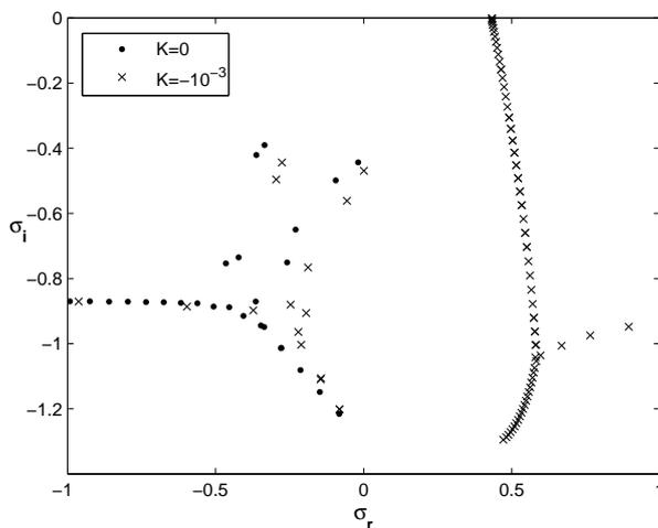
Fig. 2: Eigenspectrum for the Newtonian and SO fluid with  $Re = 2013$ ,  $\alpha = 1.3$  and  $N = 120$  at  $\gamma = 0$ .
