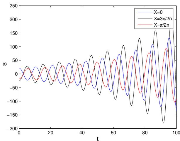
Fig. 11: Time evolution of near-wall perturbation vorticity as a function of  $x$  for Poiseuille flow ( $Re = 5000$ ,  $K = -2.10^{-3}$ ,  $\gamma = 0.03$ ,  $\alpha = 1$ ,  $\Delta t = 0.5$ ).
