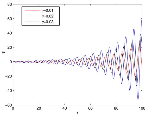
Fig. 10: Time evolution of near-wall perturbation vorticity at  $x_c = 3\pi/(2n)$  as a function of  $\gamma$  for Poiseuille flow ( $Re = 7000$ ,  $K = -10^{-3}$ ,  $\alpha = 1$ ,  $\Delta t = 0.01$ ).
