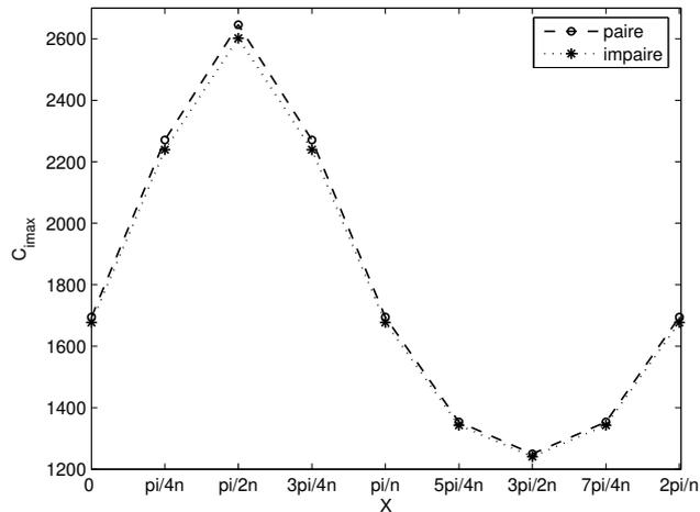
Fig. 9: Variation of the imaginary part of the most dangerous Odd and even eigenmode at different section  $x$  for SO fluid.
