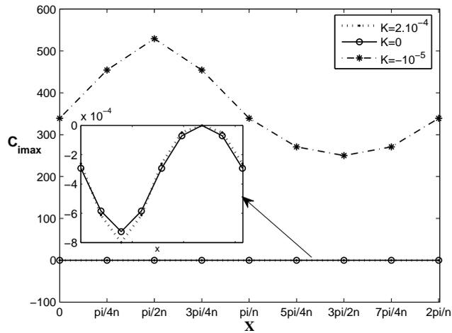
Fig. 7: Variation of the imaginary part of the most dangerous eigenmode at different section  $x$  for  $\gamma = 0.01$  and  $Re_c$  corresponding of the most dangerous section.
