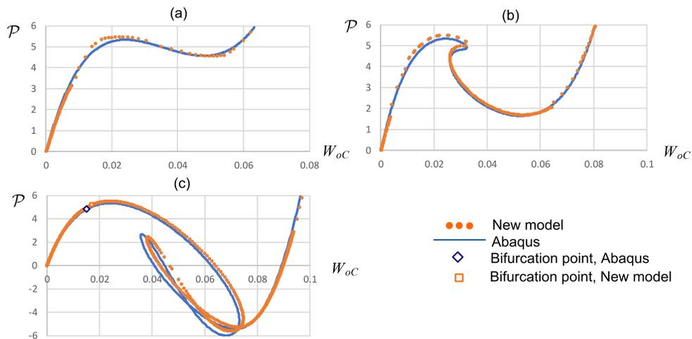
Fig. 6: The in-plane behaviour of (a) f-f, (b) p-f, (c) p-p arches when  $\vartheta = 0.3$  and  $S/r=100$
