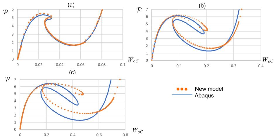
Fig. 7: In-plane behaviour of p-f arches when  $\vartheta$  is (a) 0.3; (b) 0.6; (c) 0.9 and  $S/r = 100$ .
