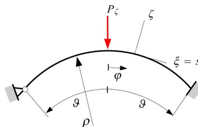
Fig. 1: The centroidal axis of a pinned-fixed arch under external load.
