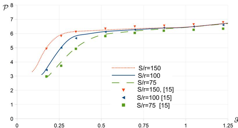
Fig. 5: Lowest buckling loads of pinned-fixed members for three  $S/r$  ratios.
