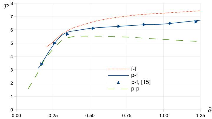
Fig. 3: Lowest buckling loads for three support arrangements,  $S/r = 100$ .
