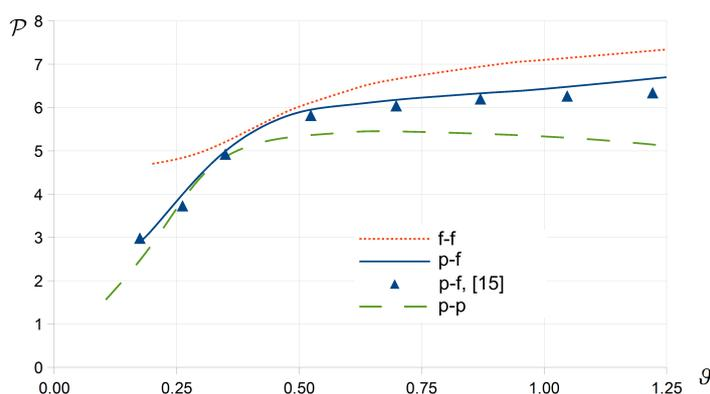
Fig. 2: Lowest buckling loads for three support arrangements,  $S/r = 75$ .
