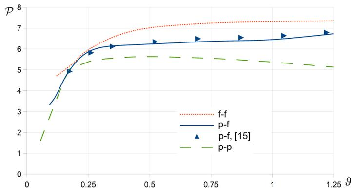
Fig. 4: Lowest buckling loads for three support arrangements,  $S/r = 150$ .
