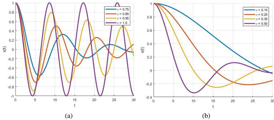
Fig. 1: Displacement of fractional oscillator under nonsingular fractional derivative operator.
