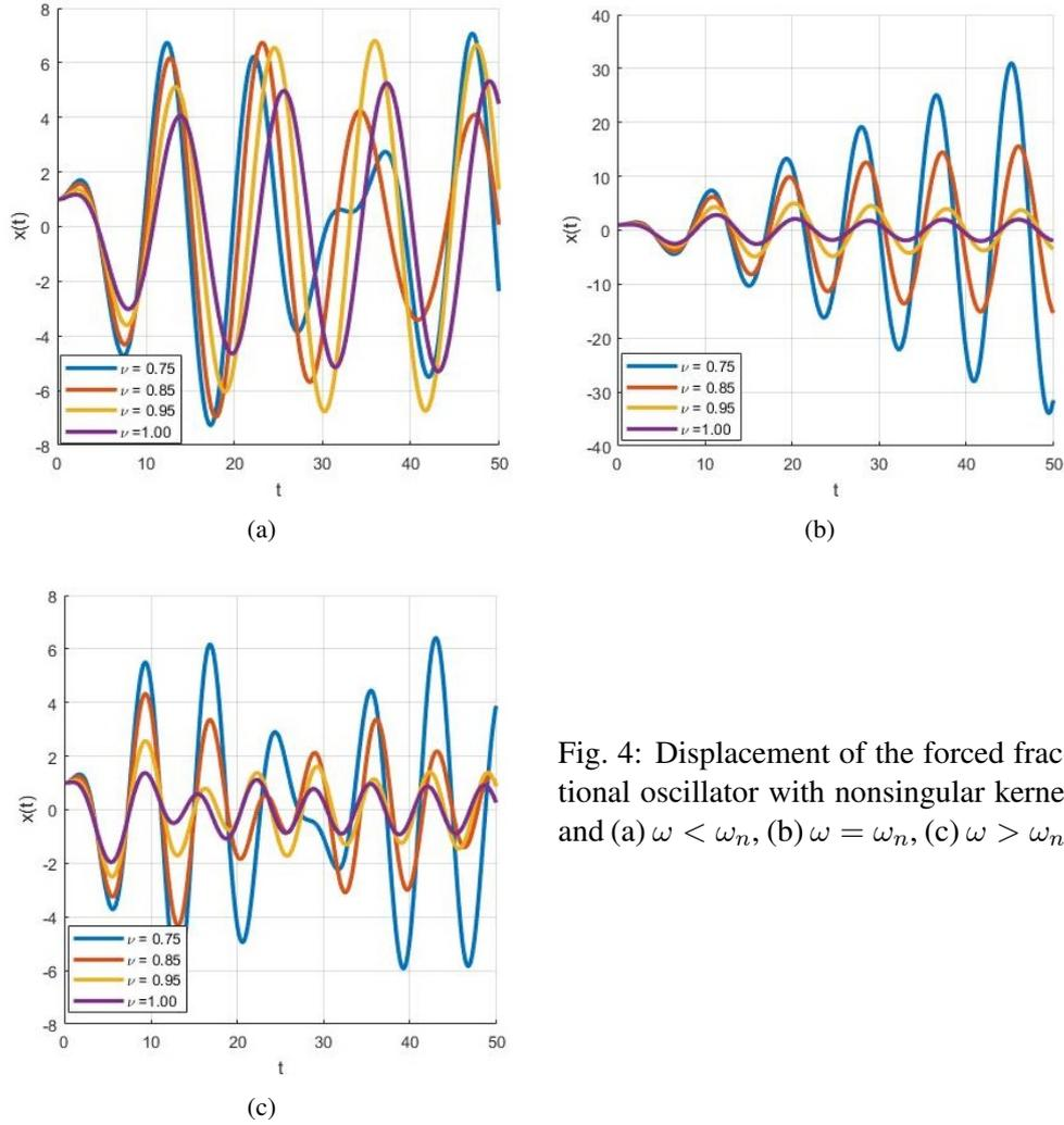
Fig. 4: Displacement of the forced fractional oscillator with nonsingular kernel and (a)  $\omega < \omega_n$ , (b)  $\omega = \omega_n$ , (c)  $\omega > \omega_n$ .
