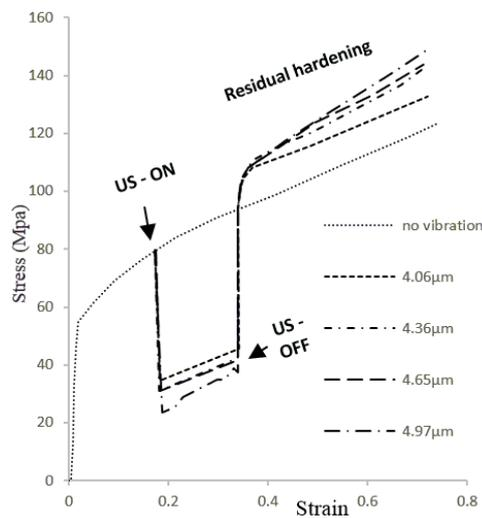
Fig. 1: Stress vs strain diagrams of aluminum in the ultrasonic field of various oscillation amplitudes [1].
