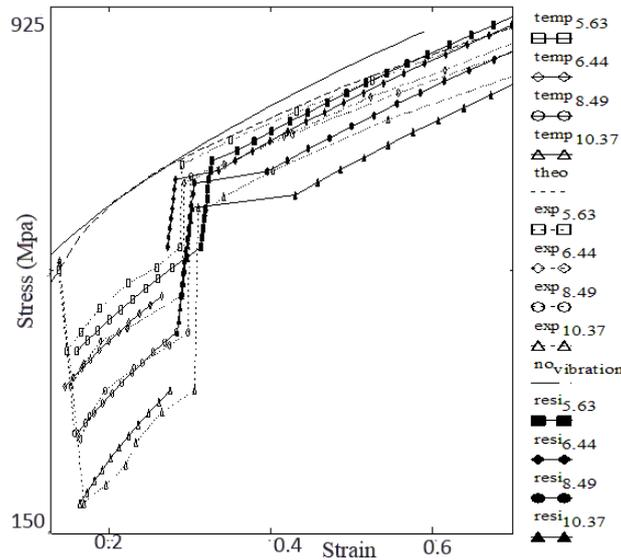
Fig. 4: Stress~strain compression diagrams of titanium in the ultrasonic field (“exp” – experimental data; “temp” and “resi” – model curves).
