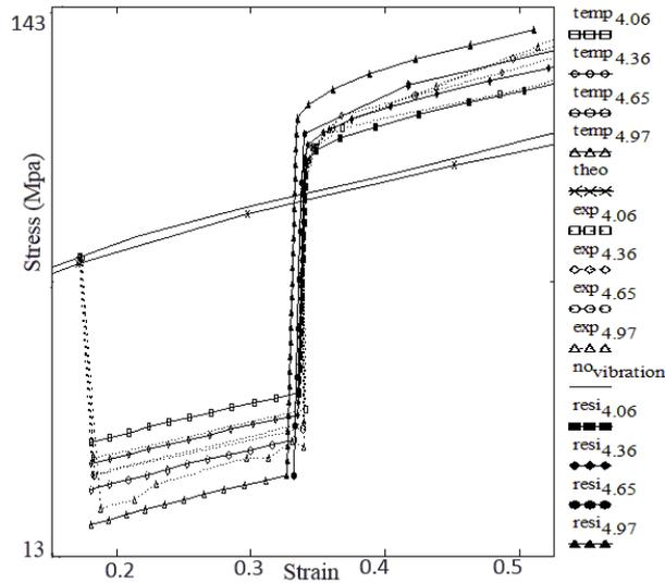
Fig. 3: Stress~strain compression diagrams of aluminum in the ultrasonic field (“exp” – experimental data; “temp“ and “resi” – model curves).
