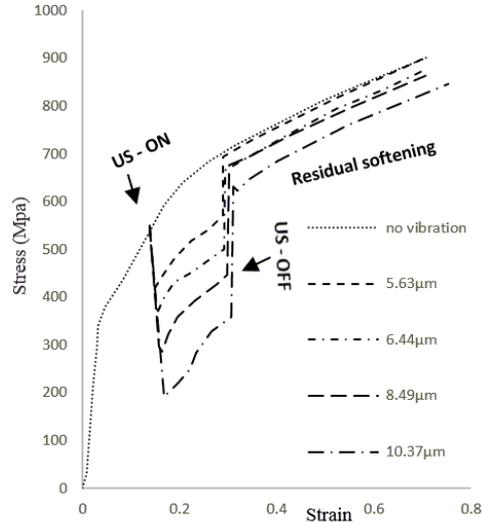
Fig. 2: Stress vs strain diagrams of titanium in the ultrasonic field of various oscillation amplitudes [1].
