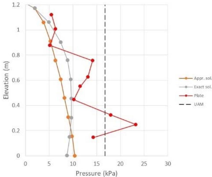
Fig. 8: Test results from Mortensen [19], and comparison with UAM theory.
