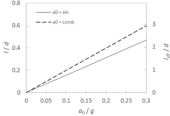
Fig. 5: Normalised added mass length  $l/d$  and effective length  $l_{\text{eff}}/d$  for constant and sinusoidally varying normalised acceleration.
