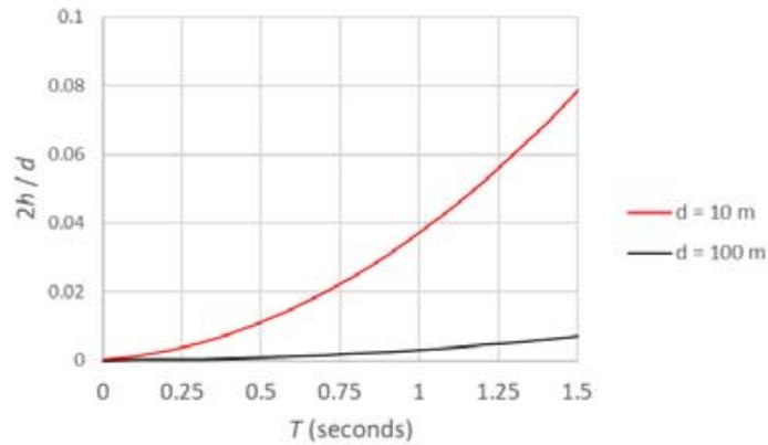
Fig. 7: Normalised WL increase  $2h/d$  as function of acceleration period  $T$ , and water depth  $d$ .
