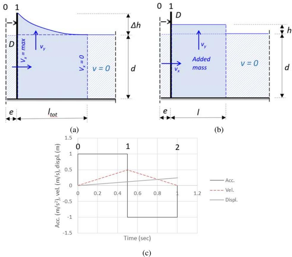
Fig. 3: Initial conditions for analysis: (a) dam displacement and water surface; (b) assumed dam displacement and uniform added mass; (c) assumed acceleration – time diagram.
