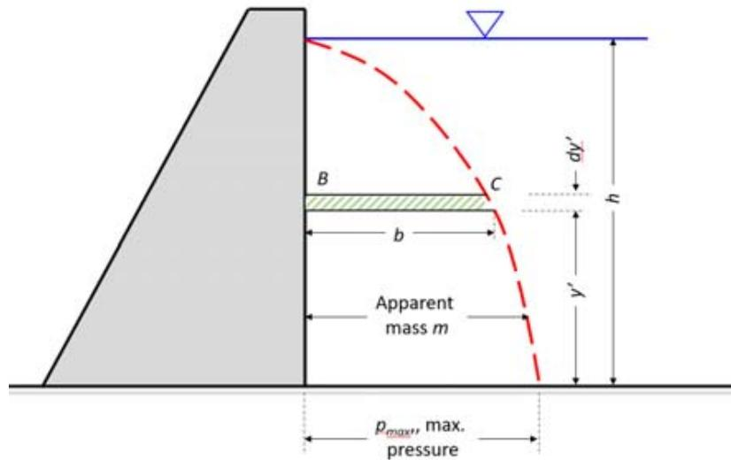
Fig. 2: Pressure distribution/added mass, [4].
