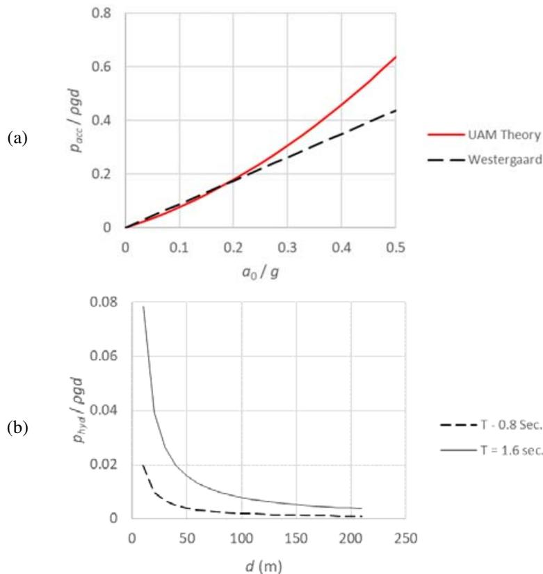
Fig. 6: (a) Normalised maximum acceleration pressure  $p_{\text{acc}}/\rho g d$ , as function of normalised acceleration. (b) Normalised additional hydrostatic pressure  $p_{\text{hyd}}/\rho g d$  as function of water depth and excitation period  $T$ .
