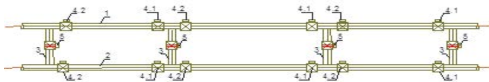
Fig. 1. Proposed schematic diagram of the parallel main gas pipeline. 1,2 - pipeline chambers on level 1 and level 2; 3 - connectors; 4.1 and 4.2 - automatic valves on pipelines; 5 - automatic valves on connectors.
